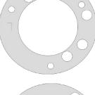
Item 7  | Copper Tube Holder Bottom & Item 13 Ring<br>Tube Bottom Hole=6mm, Dia=25mm                | 3mm   | 1pcs |
