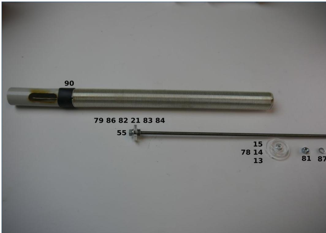
turn transport ring M4 onto the middle threaded rod
