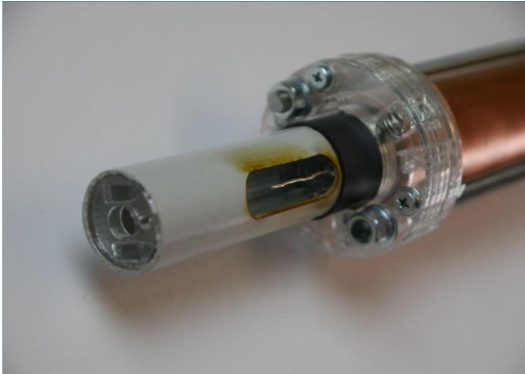
attach the silver wire to the spotlight with a cable tie. With the new spotlights a hole and the silver wire is attached there with a screw/nut.
