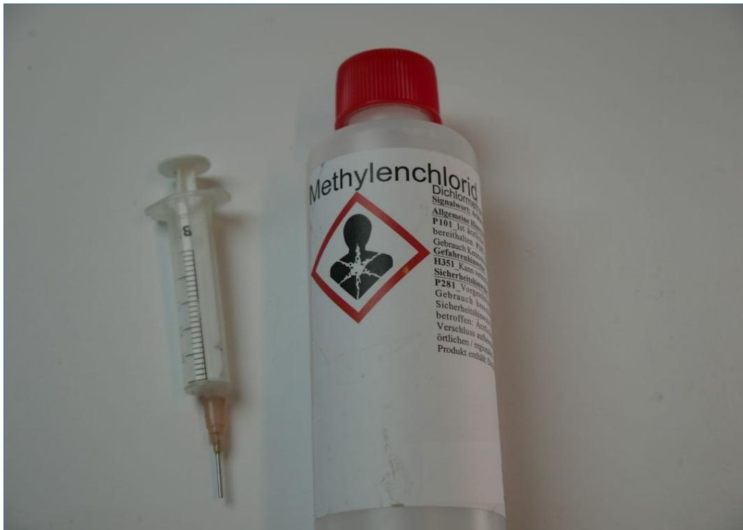
Glue the center ring (transport) with methylene chloride or acrylic glue
