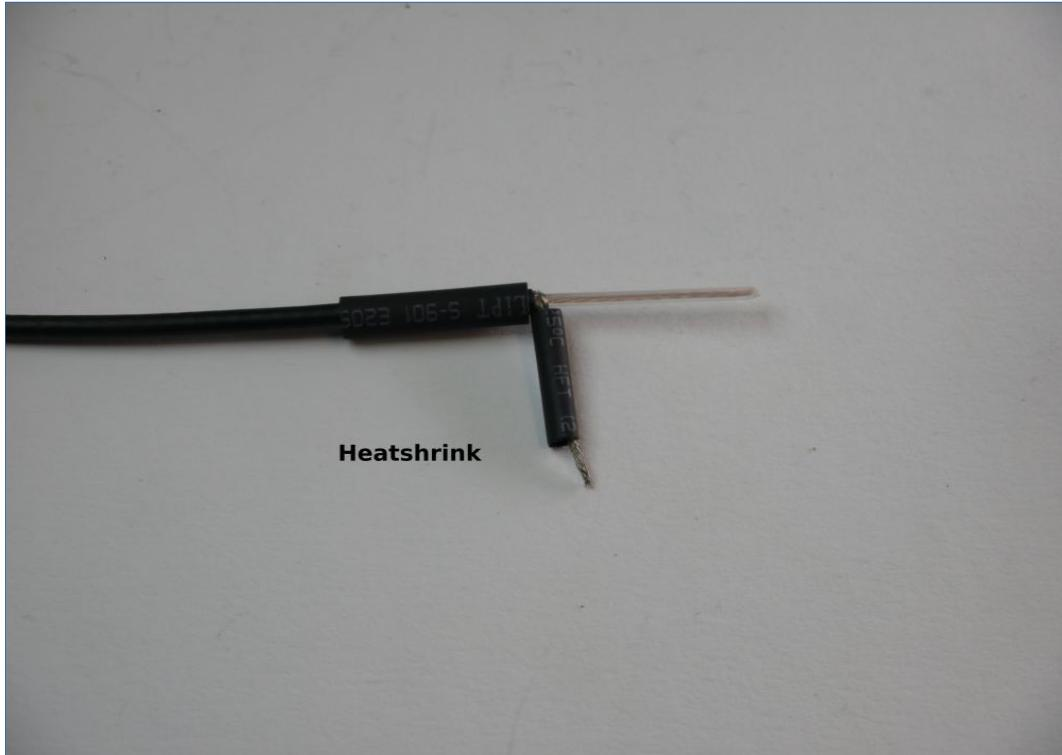
cut the inner part to approx. 5mm as shown in the picture
